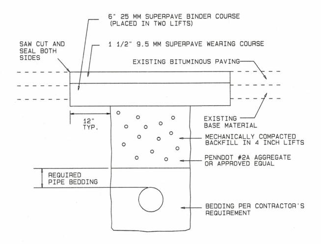
FOR USE ON OPEN CUTTING OF EXISTING BOROUGH ROADS FOR INSTALLATION OF UTILITY LINES, SEWER LINES, WATER LINES, ETC.
