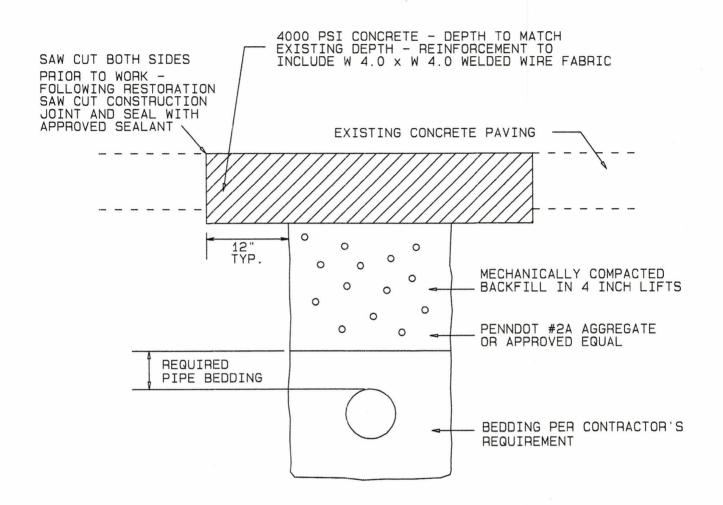
FOR USE ON OPEN CUTTING OF EXISTING BOROUGH ROADS FOR INSTALLATION OF UTILITY LINES, SEWER LINES, WATER LINES, ETC.
